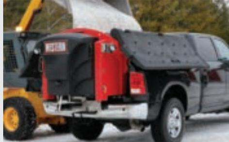
The overlapping poly hopper covers shield de-icing material from the elements, seal out moisture and act as spillguards to protect the truck from material overflow during loading.
